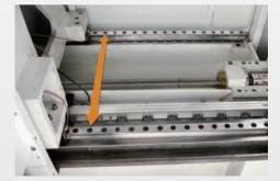
Large diameter ball lead screw and wide span Roller Guide way ensure high load capacity, low friction, and low vibration movement.
